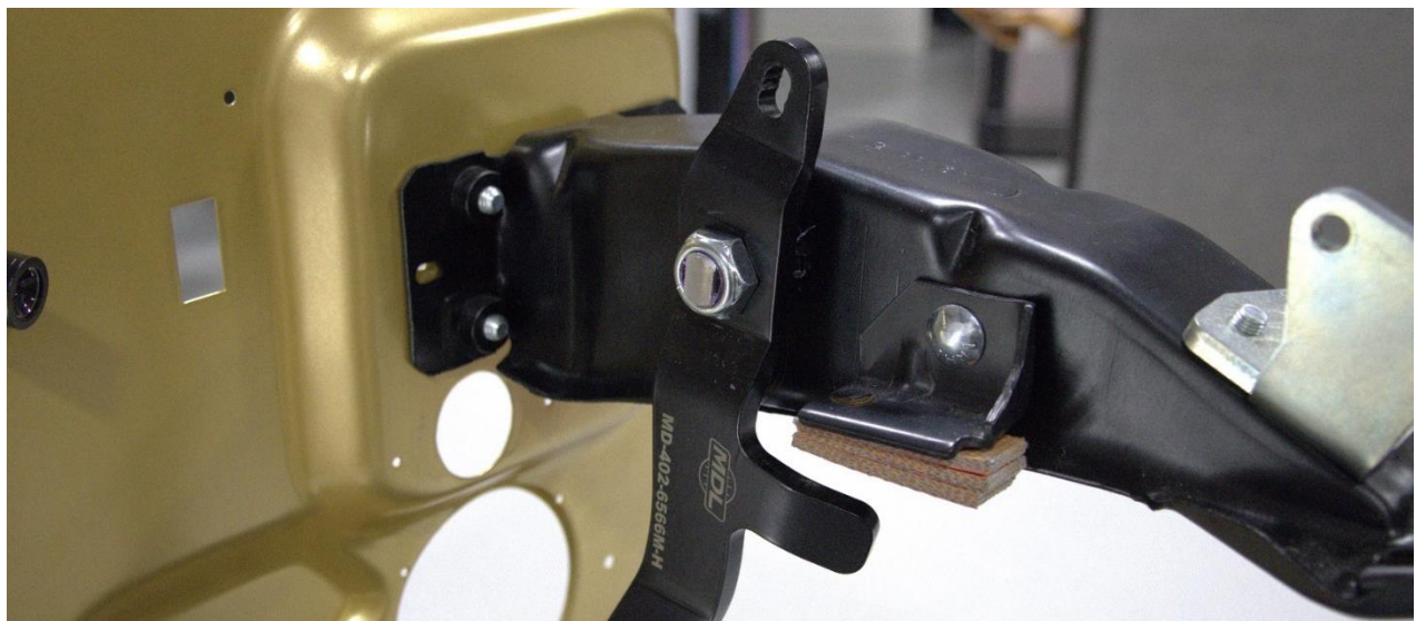
MDL supplied clutch pedal shown installed. Cylinder and brake pedal not shown for clarity.
