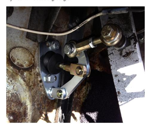
2.2 Clean surfaces of firewall and master cylinder spacer block. Apply silicone sealant to surface of block. Using a second person, Position the Master Cylinder with block through the hole and install cap screws with Loctite using a 3/16" Allen wrench. Temporarily install clevis pin and nylon washer.
