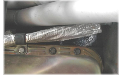
Tri-y headers shown here with the cable too close.
