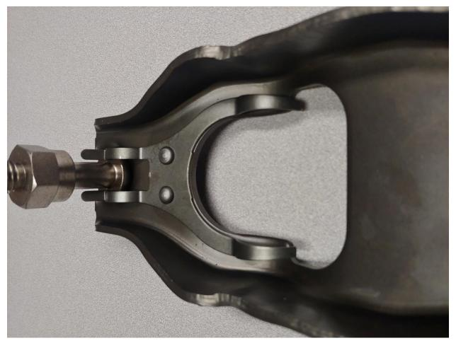
Above is the pivot stud correctly attached to the fork (not attached to the bell)
