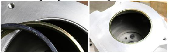
The reduction ring should slip into the opening until flush.
