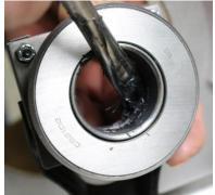
3.6Place the transmission at the edge of a bench and install the adapter to the transmission. Place the supplied throwout bearing over fork and the transmission input shaft while placing the adapter over the bearing retainer.
