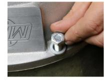
2.6 Other verification steps you can perform are "face" (mounting surface) run-out and "bore" run-out, which aid in a smooth clutch and healthy transmission bearing life. Specification is no more than .010" on the dial or .005" out of
