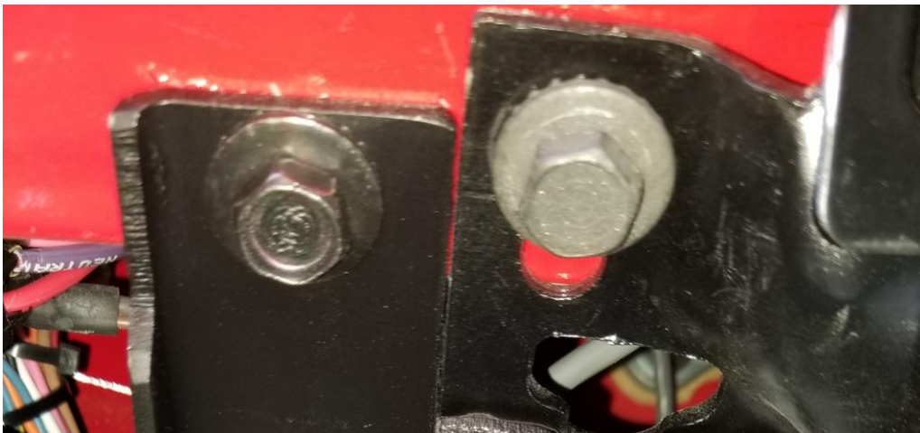
Alternate fastener shown for MDL bracket mounting next to steering column support
