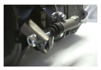
3.2 Install the socket on the aft side of the clutch lever in the inner hole and install the nut and lock washer on the front side and tighten using a 15/16" socket/wrench.
