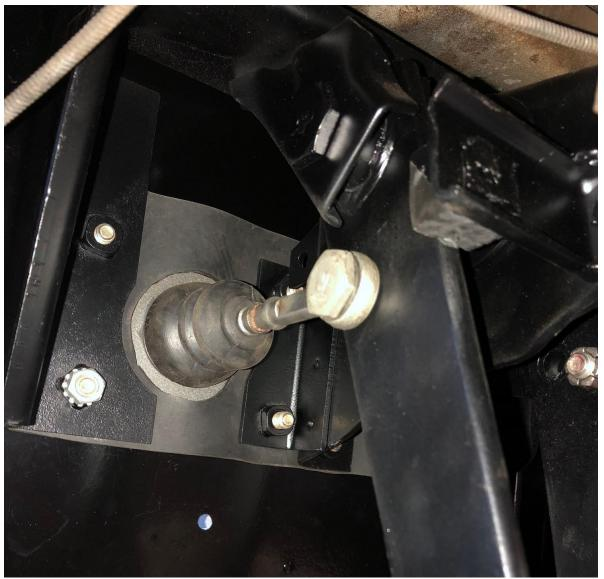
Shown is the Original Equipment clutch master cylinder bolted to the firewall and the original rod and adjusting bolt. These components will be removed and not re-used. The clutch pedal up-stop and clutch pedal will be maintained.
