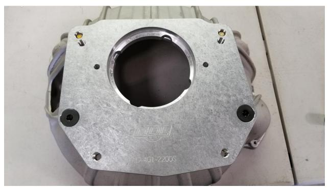
Install (4) 7/16"-14 supplied fasteners for transmission and torque to 19 ft/lbs (dry) or 15 ft/lbs with antiseize compound applied.
