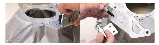
4.3 Install bracket on bell housing with 5/16" bolts and lock washers. Bracket installs INSIDE the bell housing.
