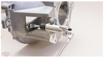
4.8 You may modify and install the clutch lever cover by trimming away the aft side of the cover to clear the slave cylinder.
