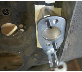
2.3 Cut out the template created in step 3.1, inside the lines, and position over the outline on the firewall. Make sure the area inside the car is clear and drill two 21/64" holes.
