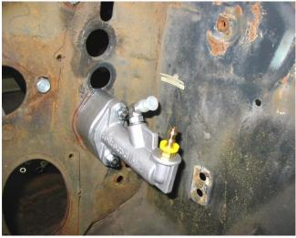
2.3 Verify actuation of the lever assy with master cylinder attached. The master cylinder will have 1.4" of total travel. Verify master cylinder does not bottom out on lever and that lever does not contact the cap screw. Install e-clip on clevis pin. Tighten the hardware as shown using a 1/2" wrench/ratchet. Verify the clutch pedal rests against the stop when adjusting rod-ends.
